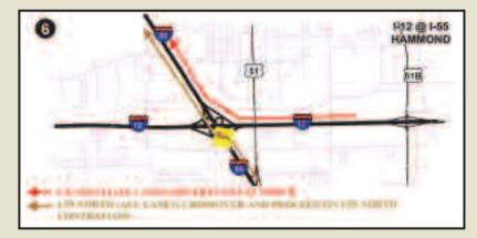
To deal with demands of traffic flow that would be created by a hurricane evacuation, contraflow freeway segments have been planned. Through use of designated contraflow points, evacuation flow is enhanced through movement of all traffic in the same direction. This diversion will enable some or all normally incoming lanes to serve as outgoing lanes to facilitate and speed evacuation.
